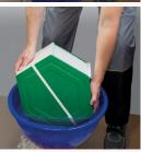
3. For added effect, fill the container with water, dip the product in the water and with smooth reciprocating movements run the water through the core (plate stack) to remove any dust, dirt or other impurities.
